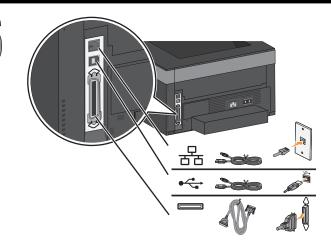
Connect the printer to a computer using a USB or parallel cable, or to a network (2330dn and 2350dn only). Cables are sold separately.
